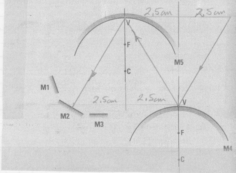
On spherical mirrors, the rays reflect such that  $\theta_i = \theta_r$ . At the vertex, V, the normal is the principle axis. Using triangles I can determine the path of the ray.
