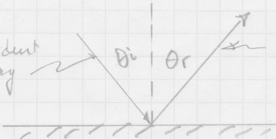
The angle of incidence equals the angle of reflection,  $Di = Or$ . These are measured between ray and the normal.
